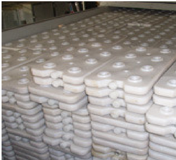
Fig. 6. PCM encapsulated in rectangular plastic containers [7].
