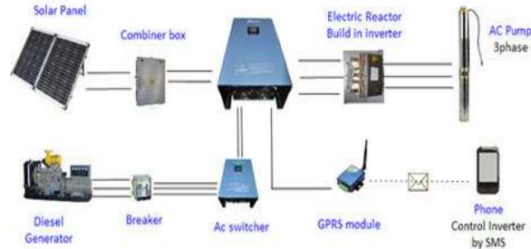
Fig. 4. Typical solar/diesel hybrid water pumping system.
