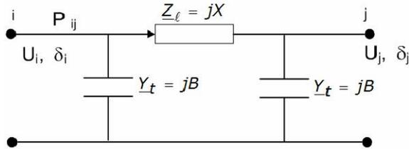
Fig. 3.  $\pi$  equivalent scheme of an electrical overhead line
