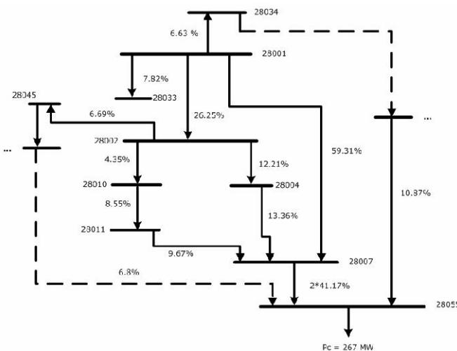
**Fig. 6. Power flow tracing for the transaction analyzed**
