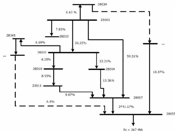
**Fig. 6. Power flow tracing for the transaction analyzed**
