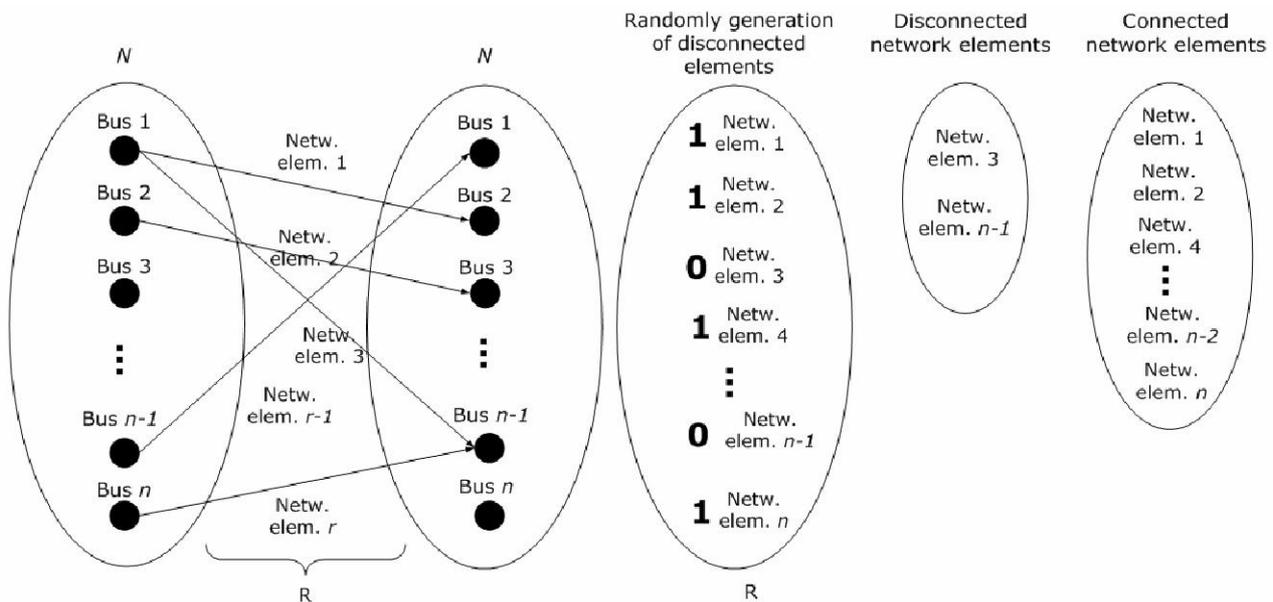
Fig. 2. The mechanism for randomly generated contingencies
