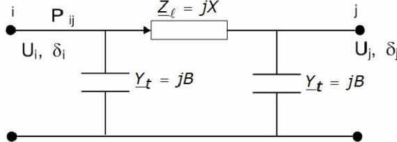
Fig. 3.  $\pi$  equivalent scheme of an electrical overhead line
