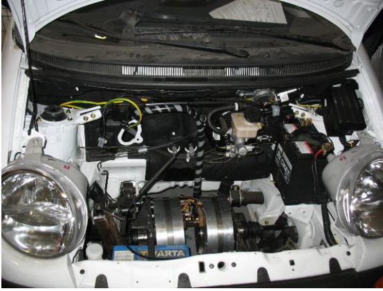
Fig. 3. The independent two-wheel drive fixed in the motor compartment
