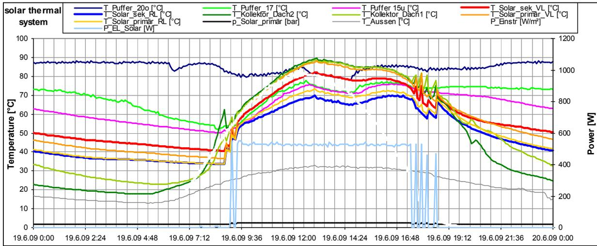
Fig. 5. Temperature and solar irradiation (P\_Einstr) of the solar thermal system on June 19th, 2009
