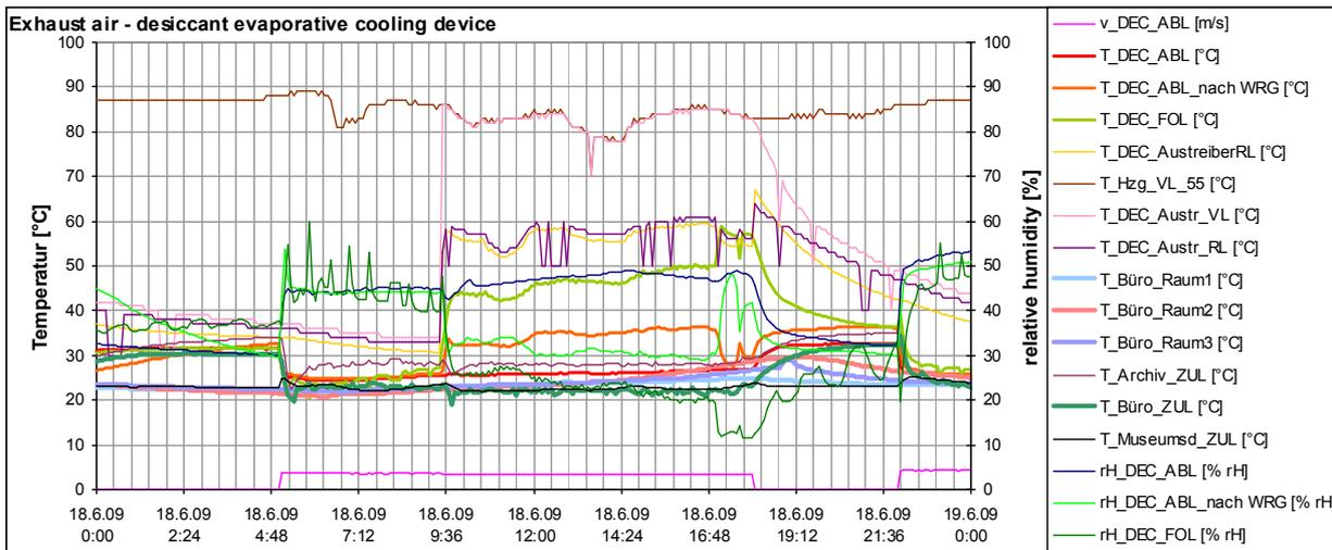
Fig. 14. DEC – exhaust air stream on June 18th, 2009
