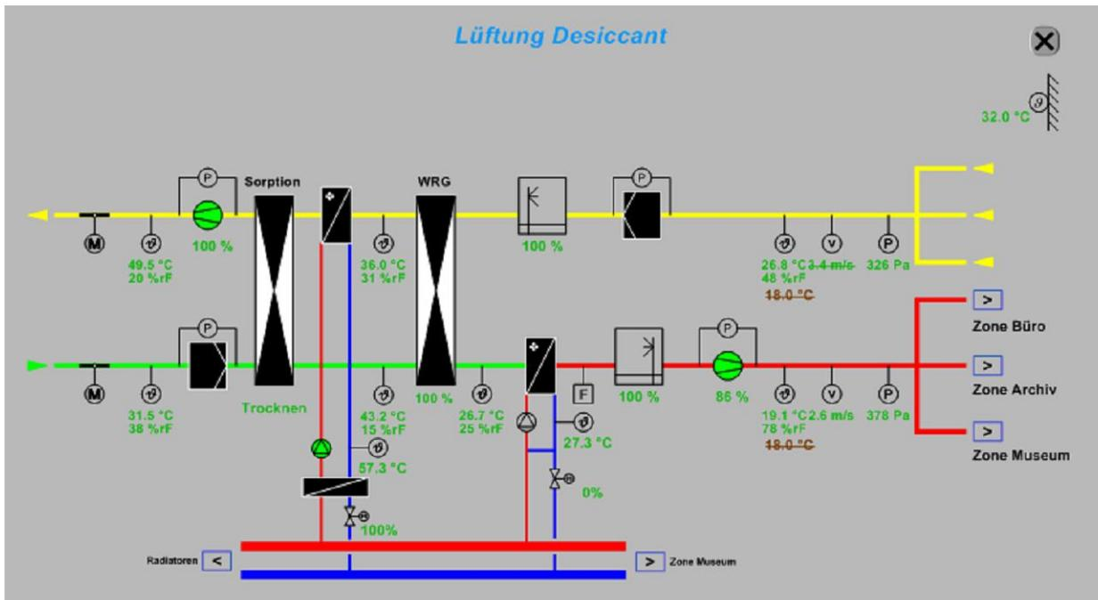
Fig. 12. Screenshot of the desiccant ventilation unit on June 19th, 2009
