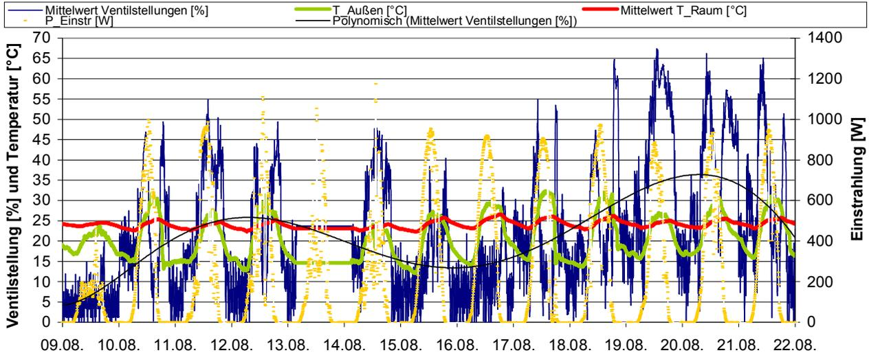
Fig. 11. Average control valve positions (Mittelwert Ventilstellungen) in relation to ambient temperature (T\_Außen), solar irradiation (P\_Einstr) and average of the 23 office room temperatures (Mittelwert T\_Raum)
