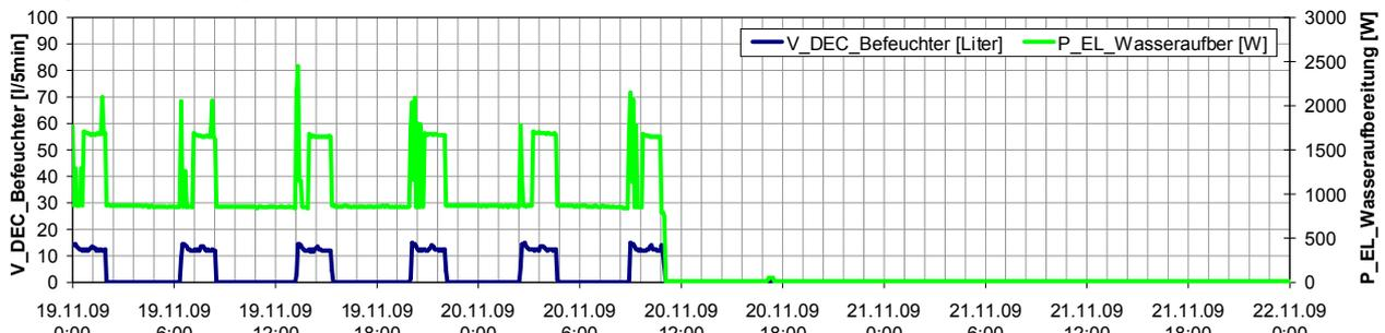
**Fig. 15. Electricity consumption (P\_EL\_Wasseraufber) and water consumption (V\_DEC\_Befeuchter) of water treatment unit before and after reprogramming**
