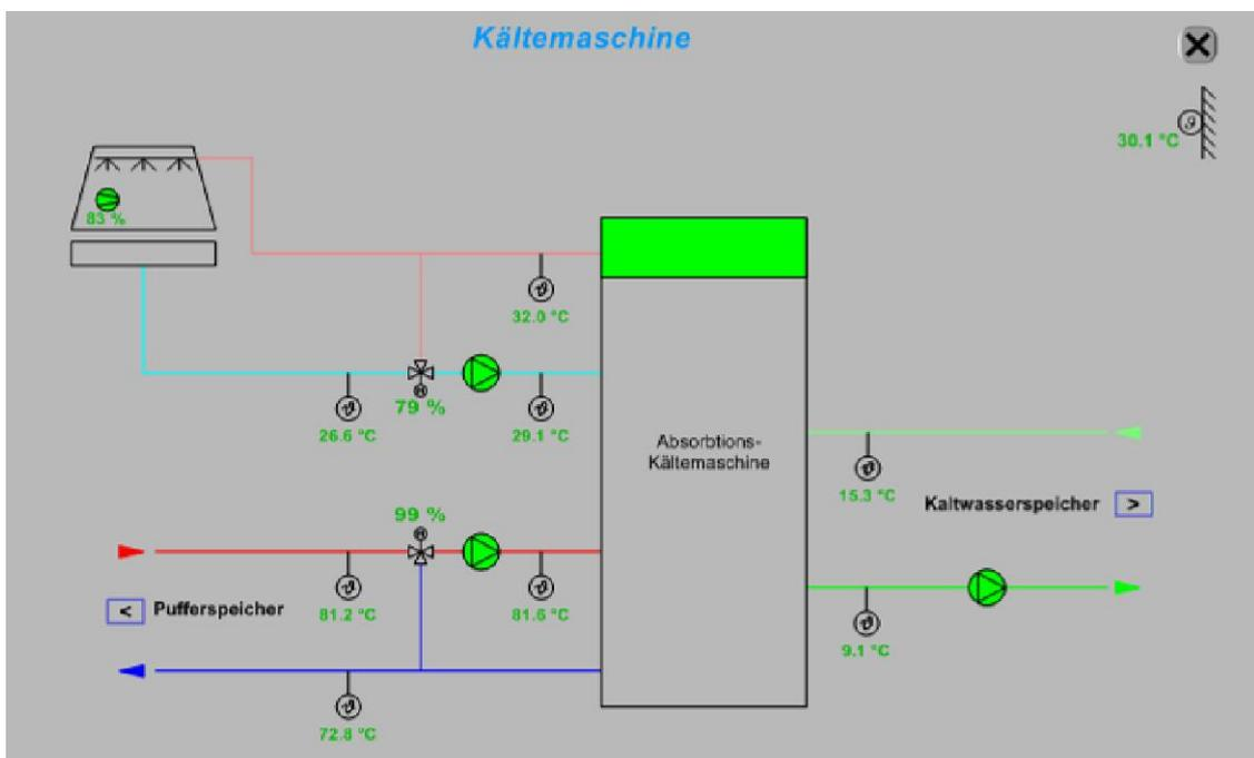
Fig. 8. Screenshot of the absorption chiller and wet cooling tower on July 30<sup>th</sup>, 2009
