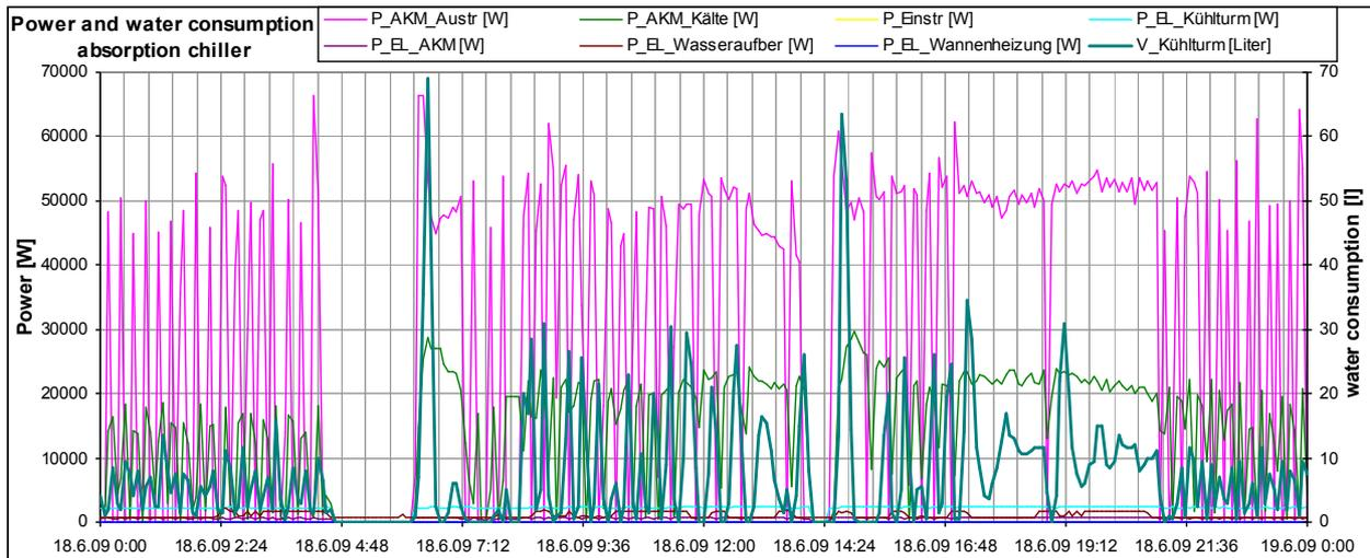
Fig. 10. Heat capacity and electrical consumption around the absorption chiller on June 18th, 2009
