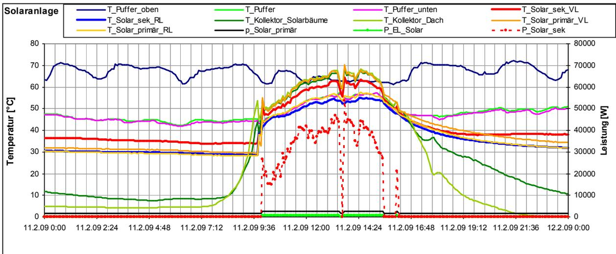
**Fig. 4. Temperature and heat capacity (P\_Solar\_sek) of the solar thermal system on Feb 11th, 2009**
