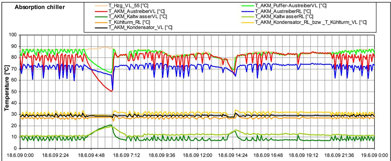
Fig. 9. Temperatures around the absorption chiller on June 18th,2009
