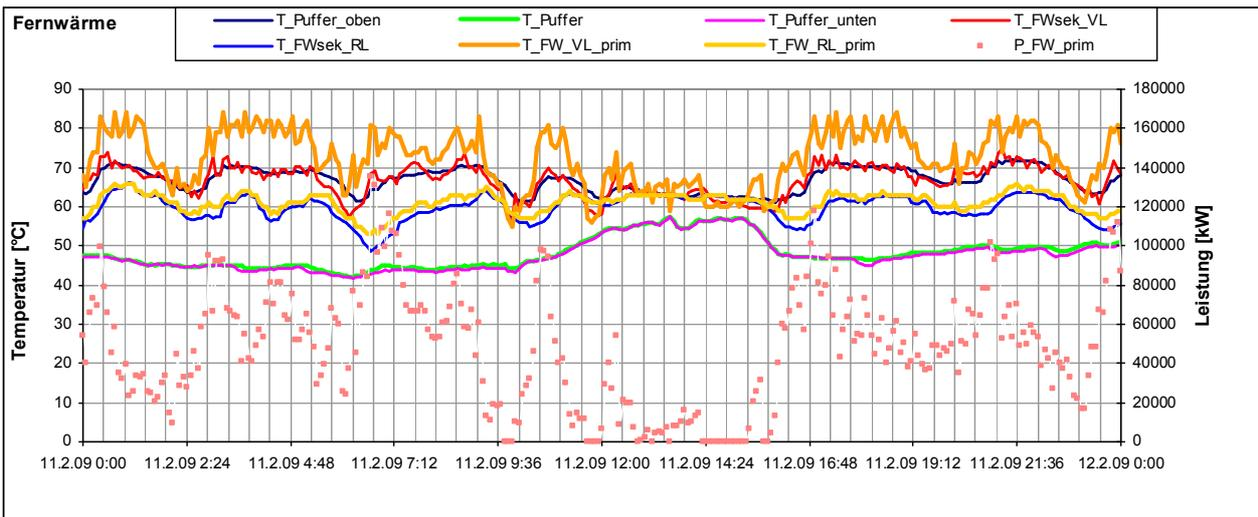
Fig. 6. Temperatures and heat capacity (P\_FW\_prim) of the hot store and the auxiliary heater on February 11th, 2009
