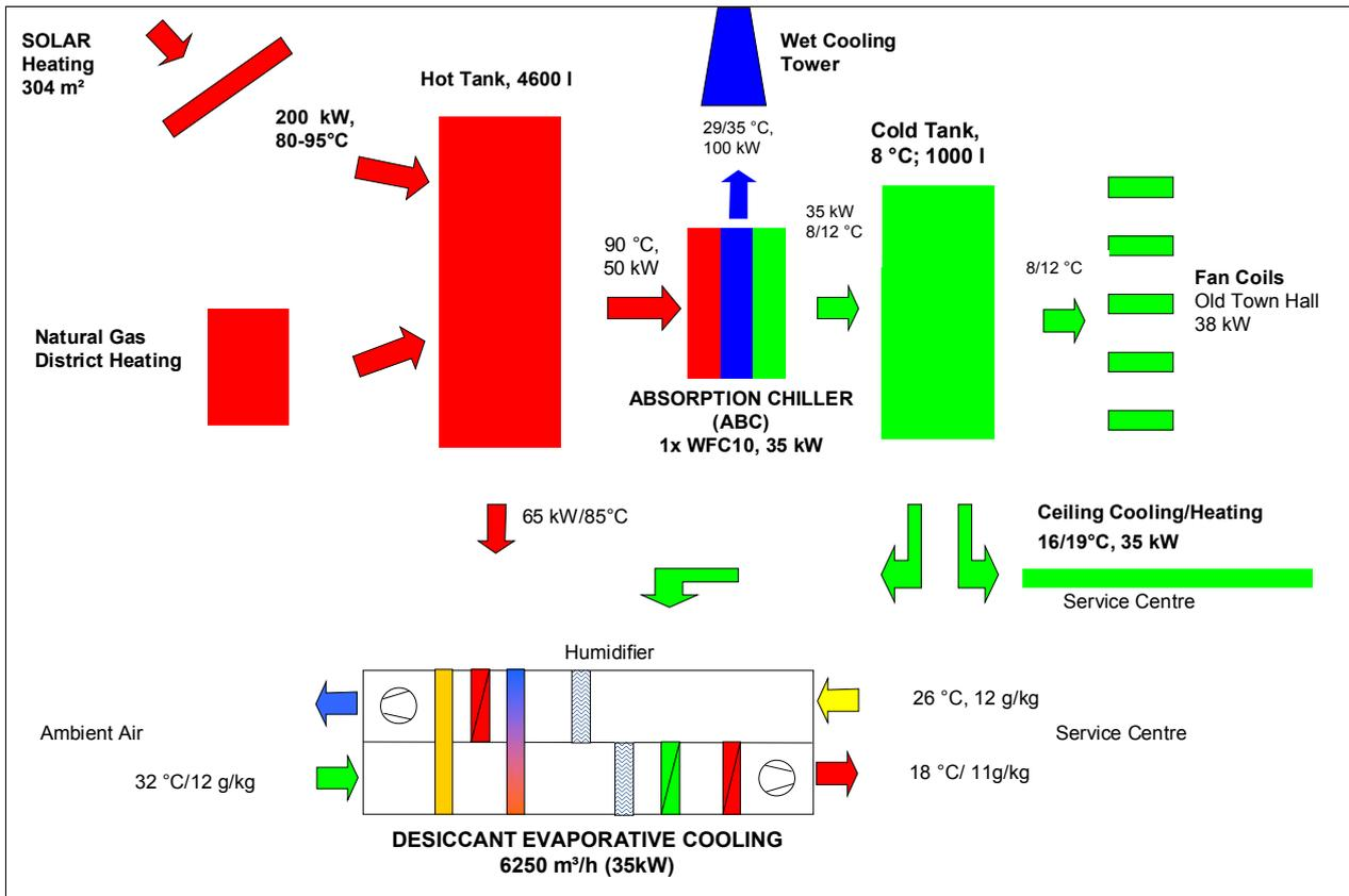
Fig. 2. Energy flow scheme of the entire system
