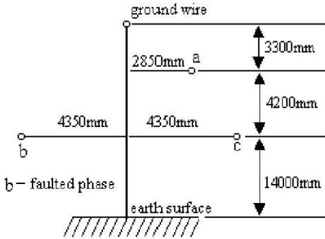
**Fig. 3 Disposition of line conductors**
