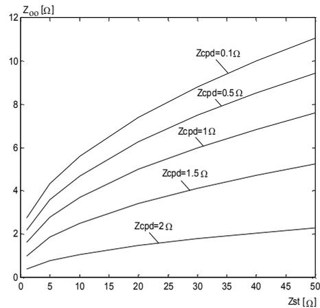
**Fig. 6 The impedance of the infinite line**
