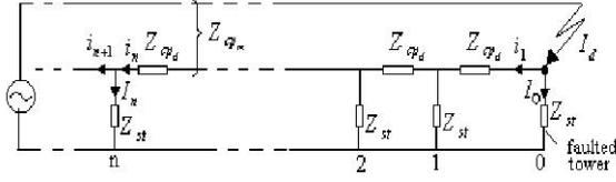
**Fig. 1 Fault current distribution**
