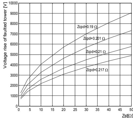
**Fig. 7 The voltage rise of the faulted tower as a function of the tower ground impedance**
