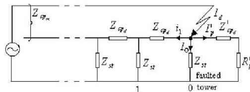
**Fig. 2 Fault current distribution**
