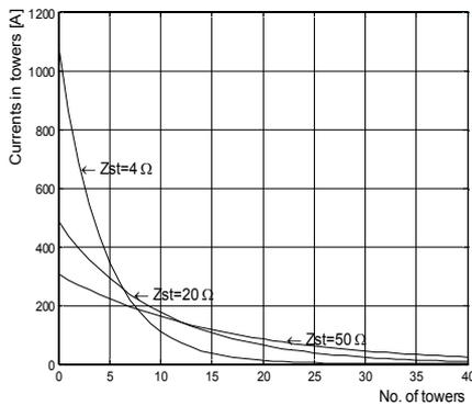
**Fig. 4 Currents flowing through the transmission line towers**
