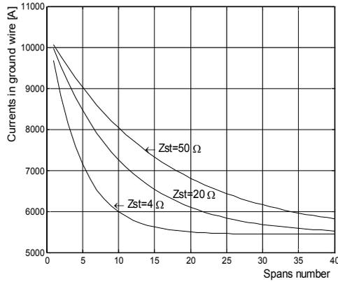
**Fig. 5 Currents flowing in the ground wire in case of different values of towers impedances**
