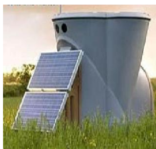
Fig. 2. Sonic device for measuring wind speed
