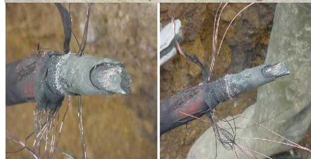
**Fig. 18. Advanced corrosion of a medium voltage cable in Cluj, due to stray currents caused by trams [24]**
