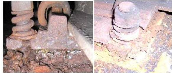
**Fig. 16. Advanced damages fixing element at underground train in Budapest (formed in about 2 years) due to D.C. stray currents**
