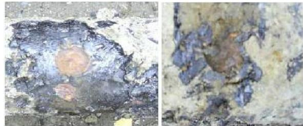
**Fig. 17. Localized corrosion on some gas pipes due to D.C. stray currents of trams and underground train in Bucharest**
