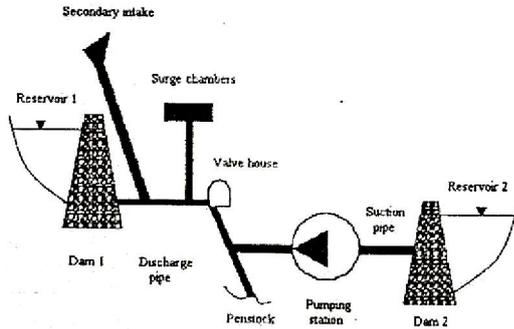
Fig. 1. The forward part of a hydro power system
