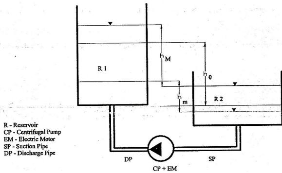
Fig. 2. Essential elements of a Hydraulic Pumping System
