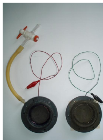
Fig. 4. Components of the microbial fuel cell used in the experiments
