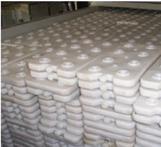
Fig. 6 - PCM encapsulated in rectangular plastic containers [7].
