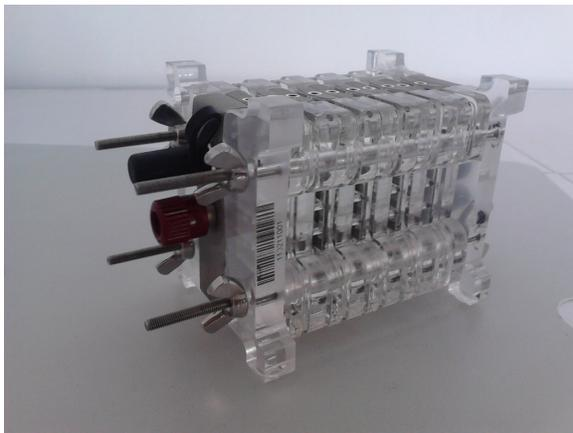
**Fig. 9 - The fuel cell stack**
