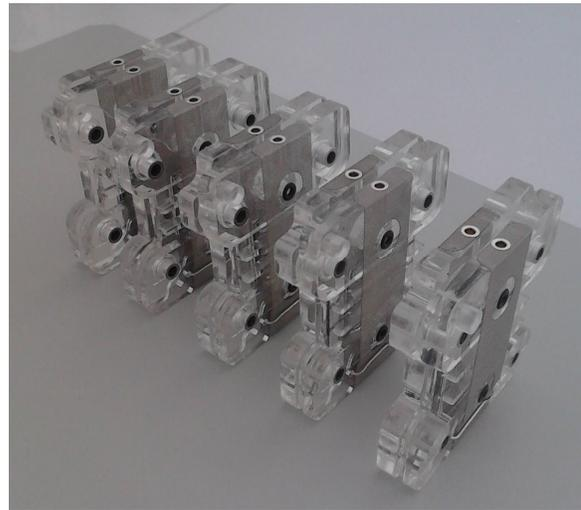
**Fig. 10 - The five fuel cells that compound the stack**
