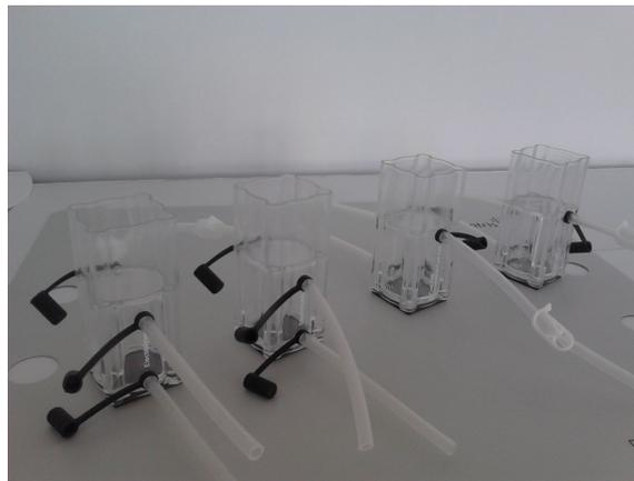
Fig. 6 - Storage canisters for hydrogen and oxygen
