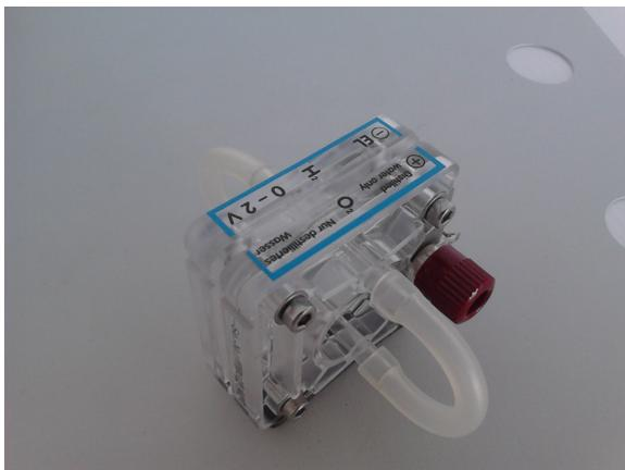
Fig. 5 - An electrolyzer used to produce hydrogen
