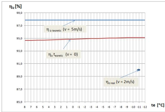
**Fig.4. The theoretic and real efficiency of the insulated flow pipe PTN**
