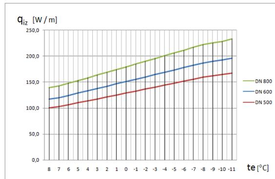
**Fig.6. Specific heat loss on DN 800, DN 600, DN 500 pipes**
