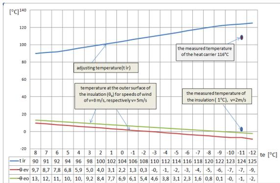
**Fig.5. The temperature at the surface of insulation (θ<sub>e</sub>) according to the calibration temperature of heat carrier (t<sub>ir</sub>) and the outer temperature (t<sub>e</sub>)**
