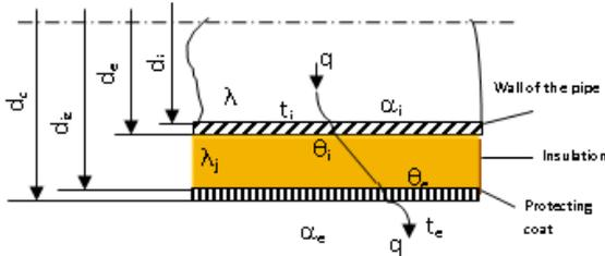
**Fig. 1. Heat transmission through the pipes**
