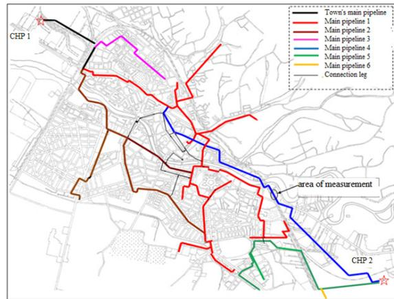
**Fig.2. Primary thermal network in Oradea municipality –Principle Scheme**
