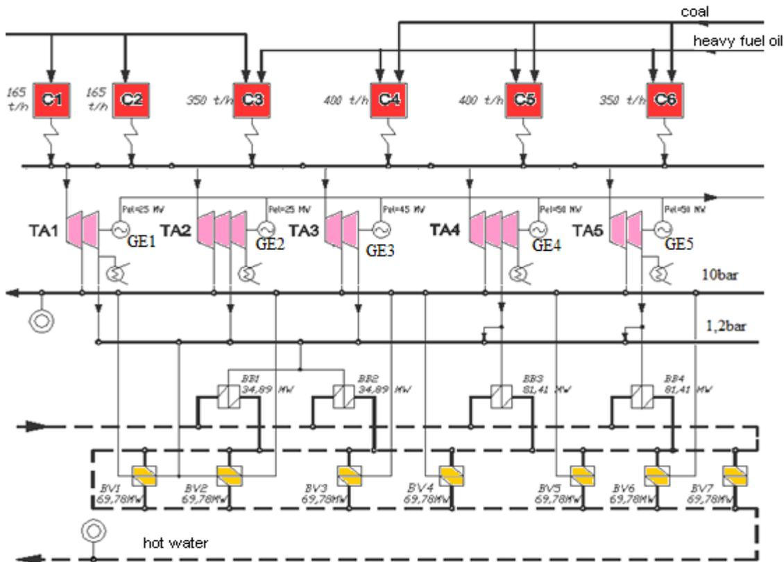
**Fig. 1. Schematic technological diagram of CHP plant Oradea**
