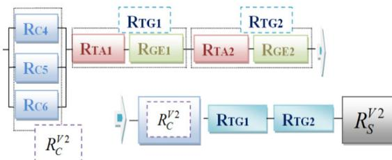
**Fig. 3. RBD of CHP plant Oradea for variant V<sub>2</sub>; R<sub>C</sub> type: „2+1” [“2 of 3”]**
