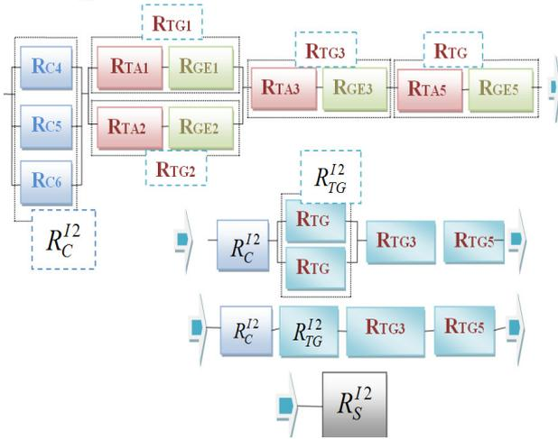
**Fig. 6 RBD of CHP plant Oradea for variant I<sub>2</sub>;**
