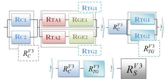
**Fig. 4. RBD of CHP plant Oradea for variant V<sub>3</sub>; R<sub>C</sub> and R<sub>TG</sub> type: „1+1” [“1 of 2”]**
