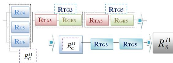
**Fig. 5. RBD of CHP plant Oradea for variant I<sub>1</sub> R<sub>C</sub> type: „2+1” [“2 din 3”]**
