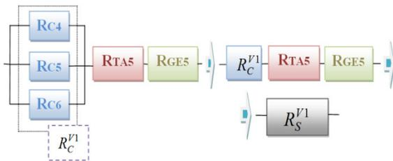
**Fig. 2. RBD of CHP PLANT Oradea for variant V<sub>1</sub>; R<sub>C</sub> type: „1+2” [“1 of 3”]**
