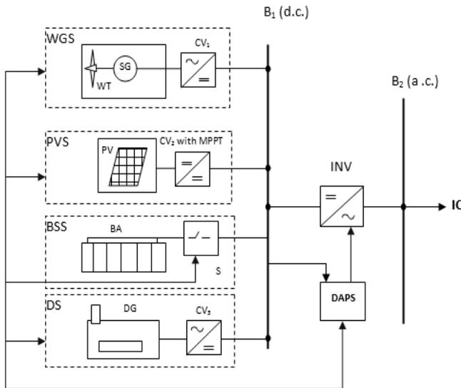
**Fig. 1. HPS block diagram utilized in reliability modeling exemplification**
