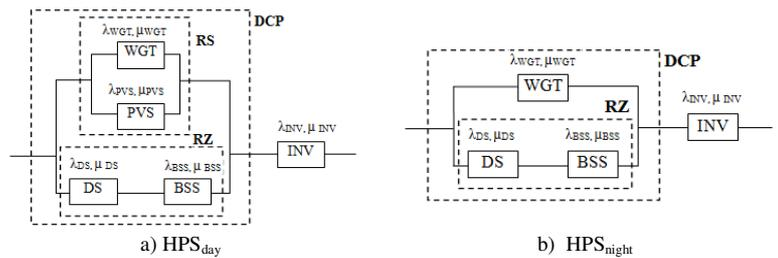
**Fig. 4. Day (a) and night (b) configuration of the HPS**
