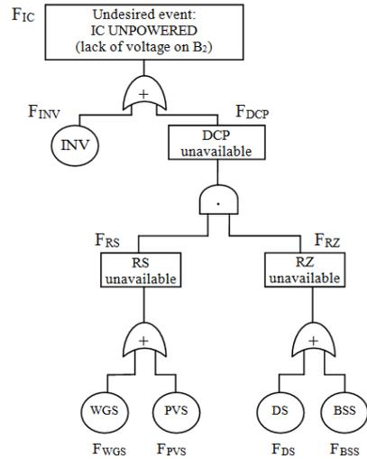
**Fig. 3. Fault three of the HPS-WSD in RZ=DS+BSS configuration**
