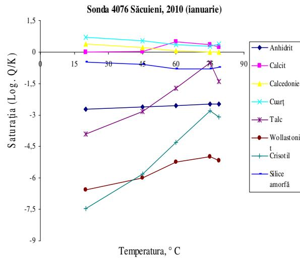
**Fig. 3. The temperature dependence of the saturation index (log Q / K).**
