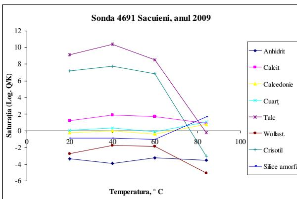
**Fig. 2. The temperature dependence of the saturation index (log Q / K)**
