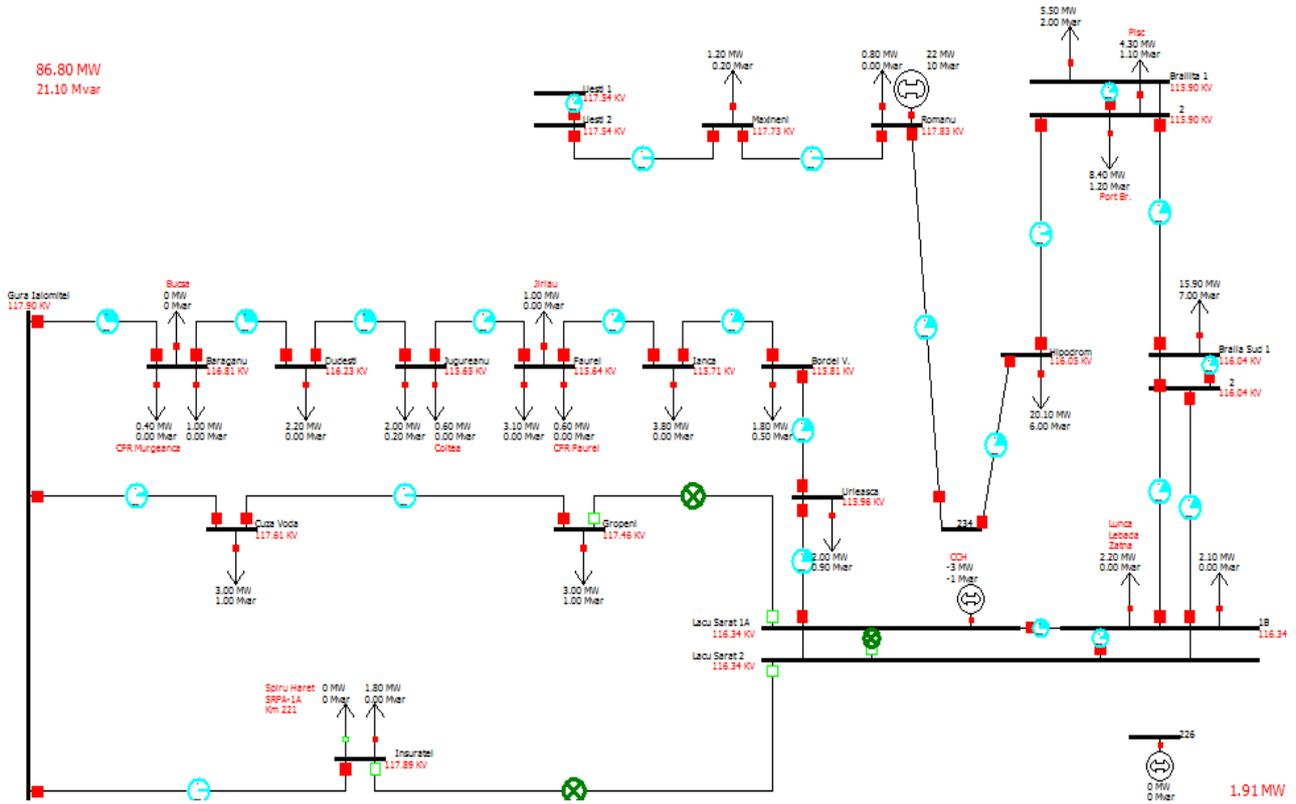
Fig. 4. Area 2 one-line diagram
