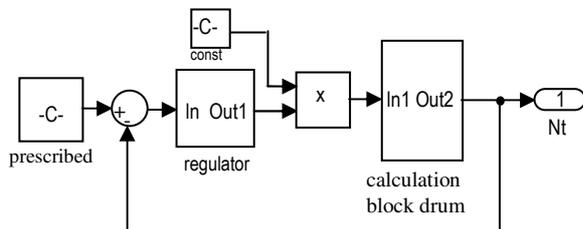
Fig. 1. Drum level control loop - current version
