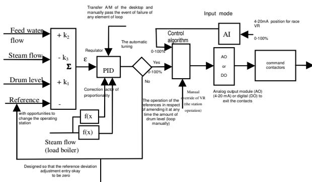
**Fig. 8. Adjustment scheme proposed – drum level, [7]**
