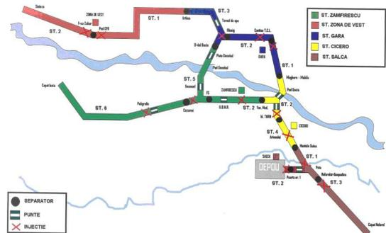
Fig. 10. Power substations and their supply network
