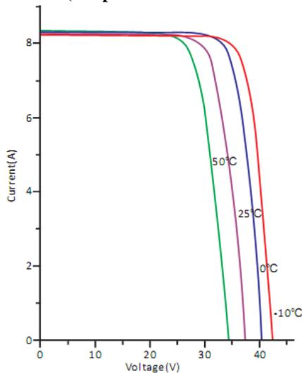
**Fig. 5 – IV Characteristics at different cell temperatures (AM 1.5, 1000 [W/m])**
