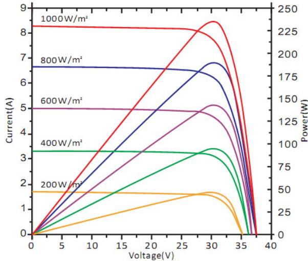
**Fig. 4 - Electrical characteristics at different irradiations (temperature is constant = 25 °C)**
