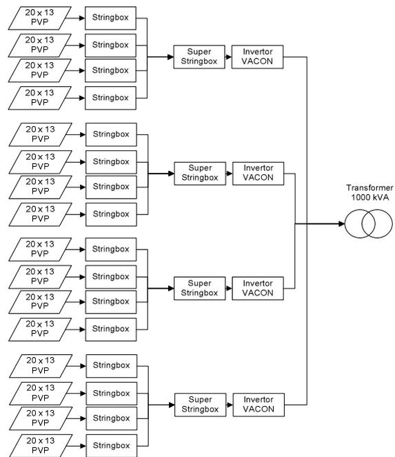
**Fig. 7 - Schematic representation of single branch connections**
