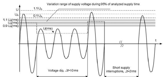
Fig. 3 – Illustration of a voltage dip and a short supply interruption
