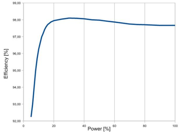
**Fig. 6 – Central inverter efficiency curve**
