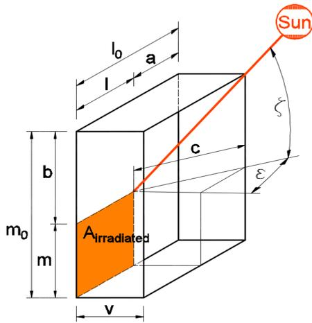
**Fig. 4. Interpretation of altitude and azimuth angles for the insolated area for given window sizes**
