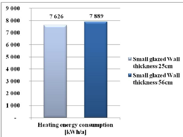
Fig. 13. Heating energy consumption of the building in function of the wall thickness– small glazed ratio
