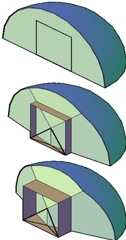
Fig 9. Solid angle intervals in which the diffuse radiation hits the glazing for different reveal depths.
