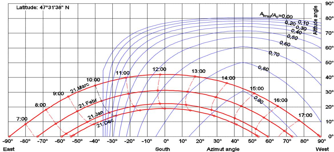
Fig. 8.  $A_{ir}/A_0$  ratio in case of wall thickness 25 cm on the sun-path diagram - orientation South-West, opening 1,5 x 1,5 m
