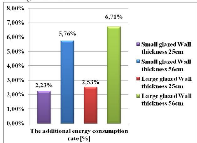
Fig. 16. The additional energy consumption caused by the reveal
