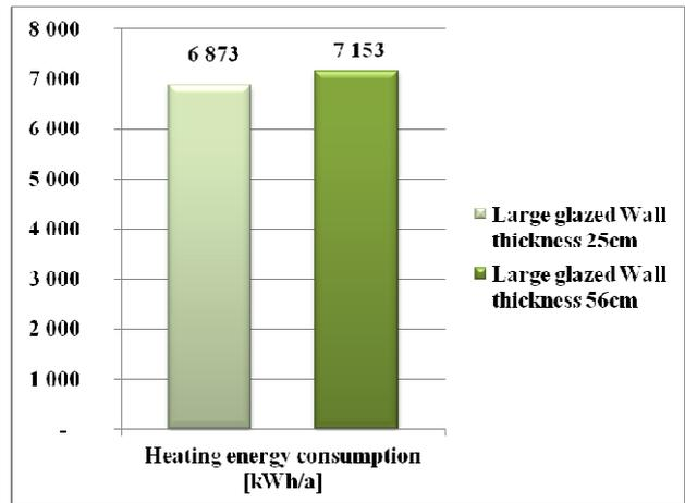
Fig. 14. Heating energy consumption of the building in function of the wall thickness reveal depths–high glazed ratio
