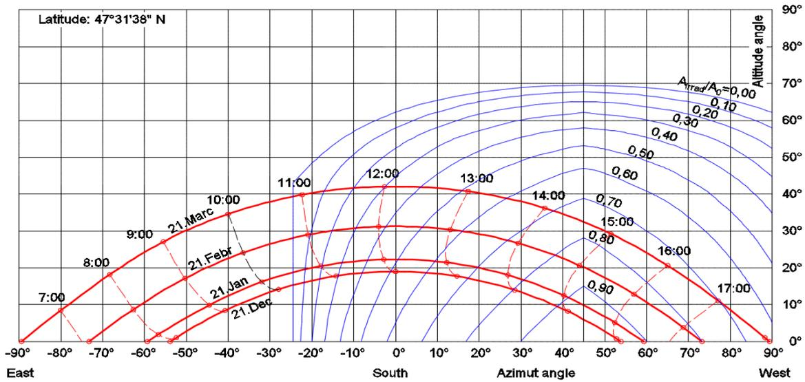
Fig. 7.  $A_{ir}/A_0$  ratio in case of wall thickness 56 cm on the sun-path diagram - orientation South-West, opening 1,5 x 1,5 m
