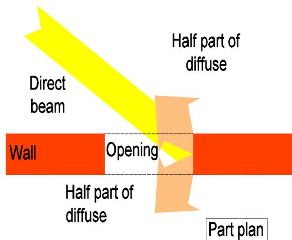
Fig. 11. Half of the radiation hitting the reveal is reflected to the glazing in case of beam solar radiation.
