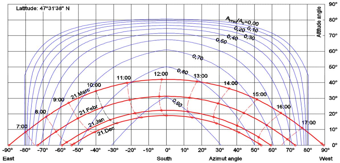
Fig. 6. The  $A_{ir}/A_0$  ratio in case of wall thickness 25 cm on the sun-path diagram – orientation South opening 1,5 x 1,5 m
