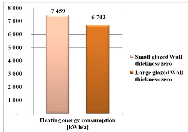
Fig. 15. The theoretical extreme heating energy consumption with zero wall thickness
