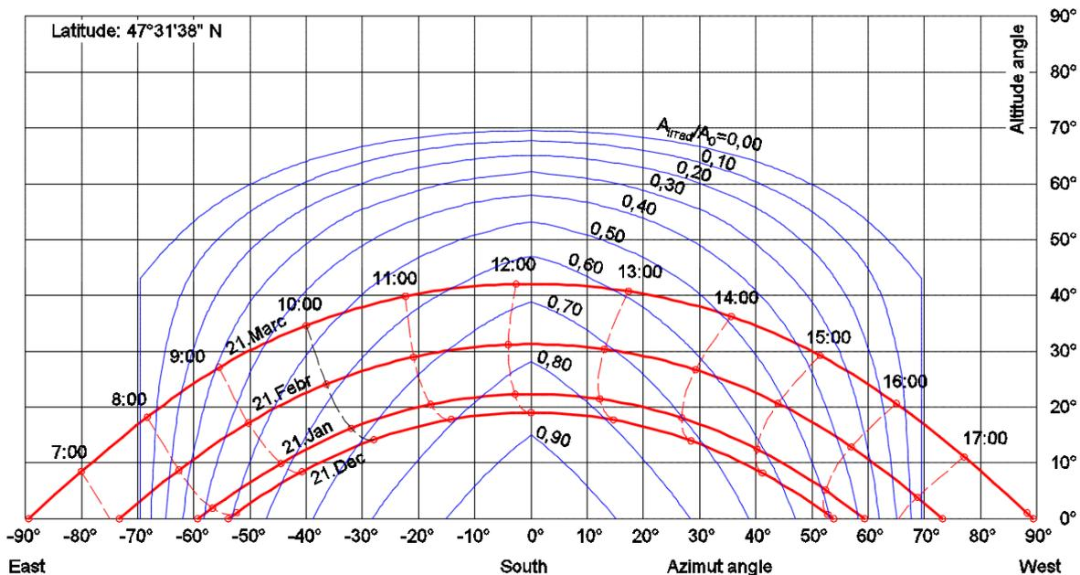
**Fig 5. The  $A_{ir}/A_0$  ratio in case of wall thickness 56 cm on the sun-path diagram – orientation South, opening 1,5 x 1,5 m**
