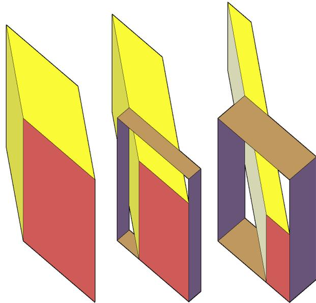
**Fig. 3 Insulated area  $A_{ir}$  in the plane of the internal wall surface show the “cross section” through which the direct beam enters the room. Its ratio to the area of the opening  $A_0$  (measured on the outer surface) shows the diminuation effect due to the reveal.**
