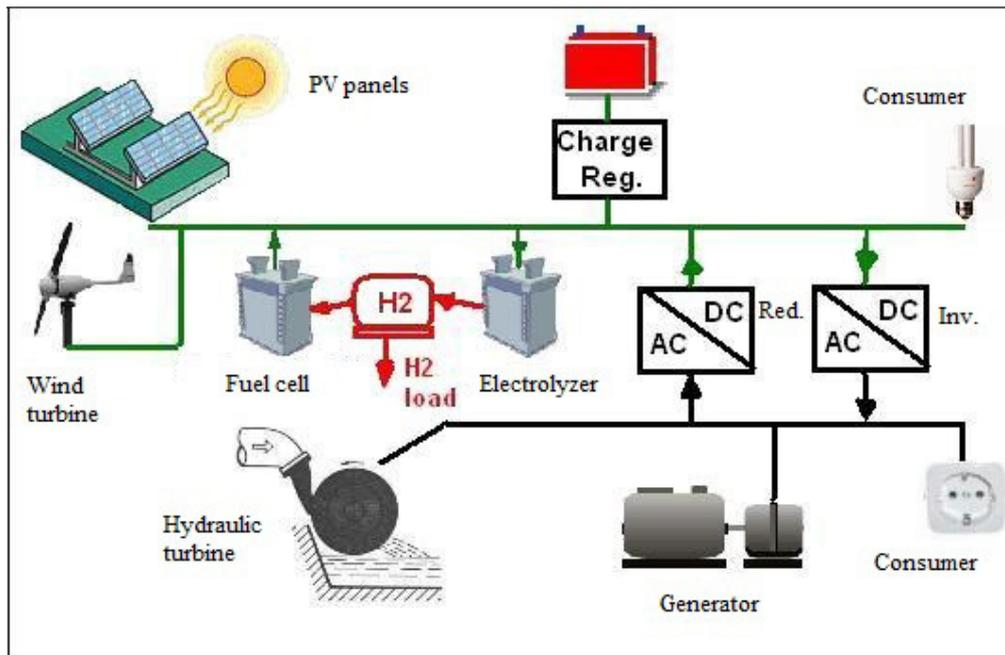
**Fig.1. Scheme of an autonomous hybrid system**
