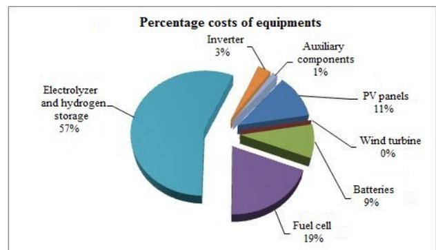
**Fig. 2. Percentage costs of equipments before the optimization of the hybrid system**
