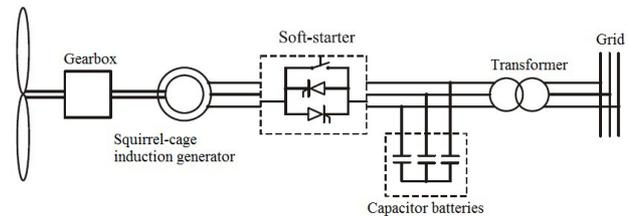
**Fig.1. Wind turbine type A - fixed speed (the Danish concept).**
