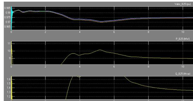
Fig.5. Grid operation with compensator STATCOM connected
