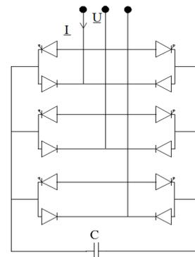
**Fig.2. Three-phase scheme of STATCOM**
