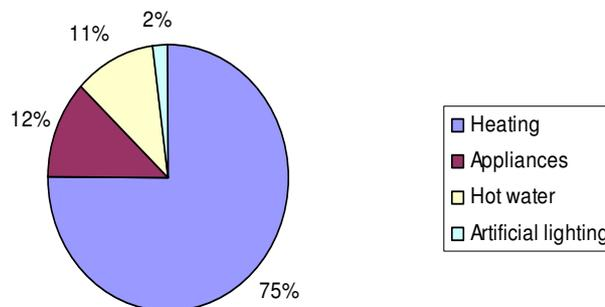
**Fig. 1. The percentage of energy consumption for a residential building in Romania**
