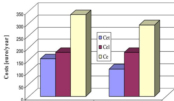
**Fig. 5. Energy costs before and after thermal rehabilitation [euro/year]**
