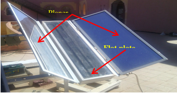
Fig.3 - Image of the prototype flat plate solar water collector with reflectors
