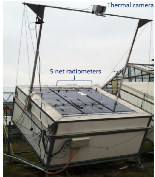
Fig. 1 - Thermal box setup for solar radiation measurements
