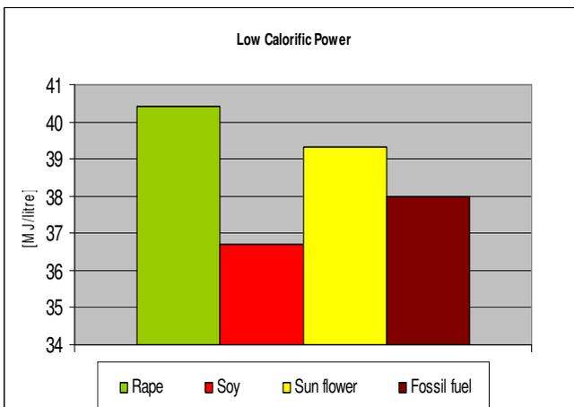
**Fig. 4 - Low Calorific Power of Bioliquids and Liquid Fossil Fuel**
