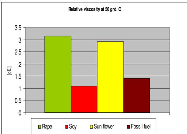
**Fig. 3 - Relative Viscosity at 50<sup>o</sup>C of Bioliquids versus Liquid Fossil Fuel**
