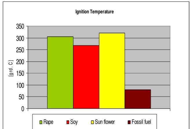
**Fig. 5 - Ignition Temperature of Bioliquids versus Liquid Fossil Fuel**
