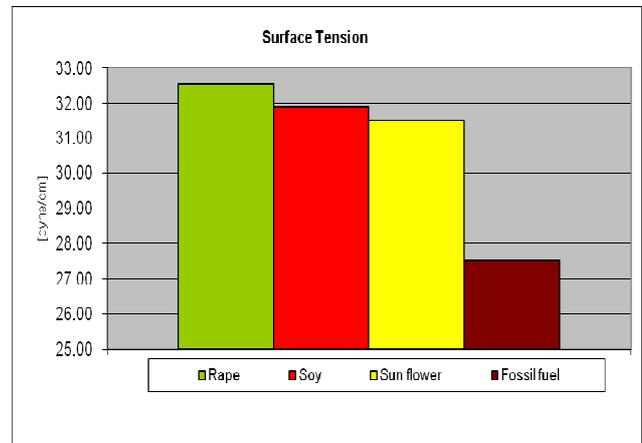
**Fig. 6 – Surface Tension of Bioliquids and Liquid Fossil Fuel**
