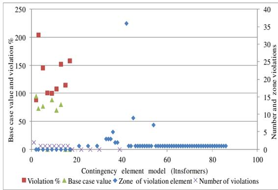
**Fig.2. Violated and contingency elements (transformers) in the power system of Kosovo**
