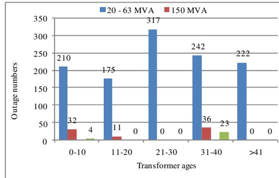
**Fig.5. Power transformers outages in the Transmission Power System of Kosovo**
