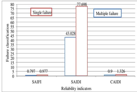
**Fig.13. Monitoring transformer reliability indicators by modeling failure mode (single and multiple)**
