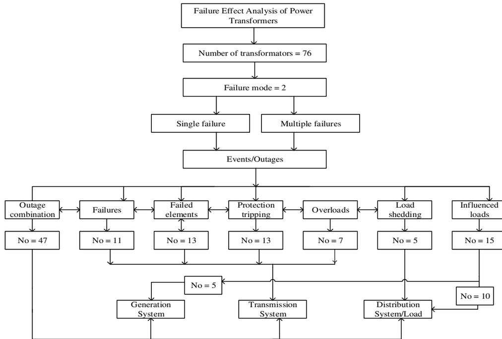
Fig.12. Failure effect analyses of the power transformers in KOSTT during the year 2016, simulated by NEPLAN
