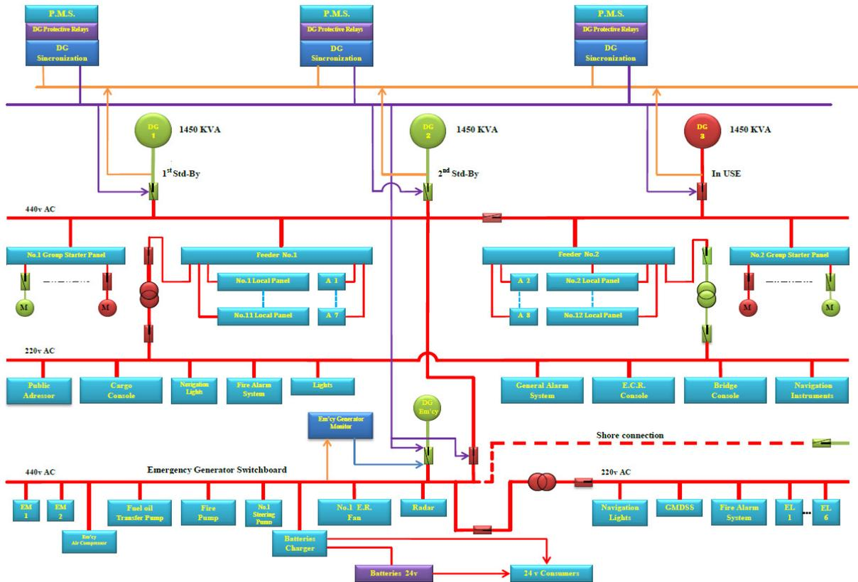
Fig. 5. The typical diagram of the SEPS' s
