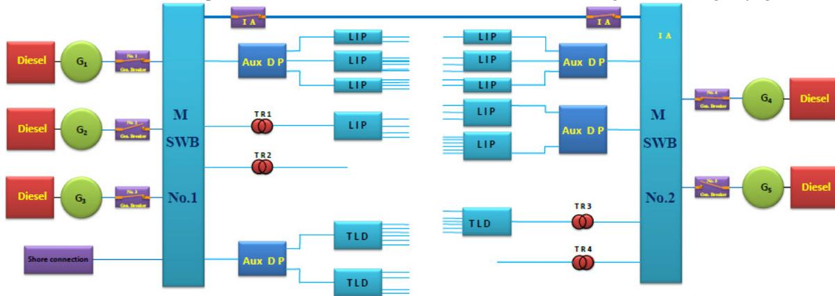
Fig. 2. Block diagram of SEPS with two main switchboard
