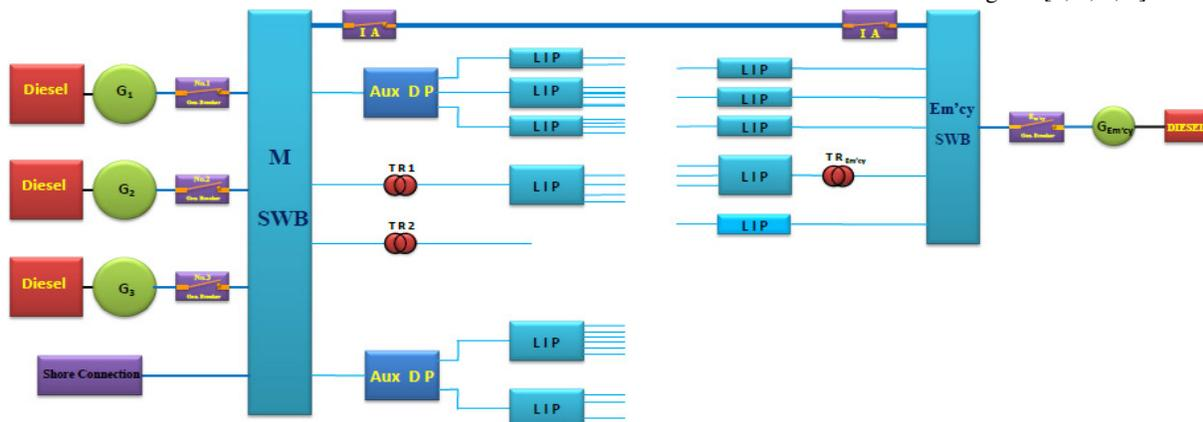
Fig. 1. Block diagram of SEPS with a single main switchboard and an emergency generator
