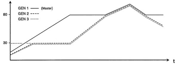
Fig. 8. Diagram of asymmetrical load distribution between generators
