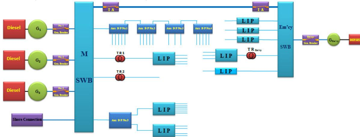
Fig. 4. Block diagram of SEPS where the electrical power distribution is done both by main lines and radial lines.
