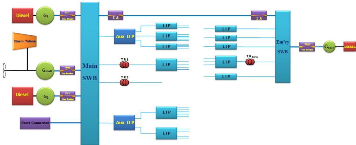
Fig. 3. Block diagram of SEPS with energy retrieval from the propeller plant by shaft generator and exhaust heat/recovery boiler
