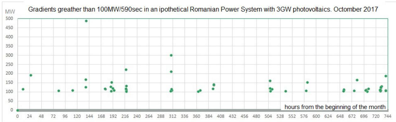
Figure 10. In an hypothetical SEN, with 3Gw insted of 1,3GW photovoltaic generators wind and photovoltaic peaks greater then 100MW inside 590seconds
