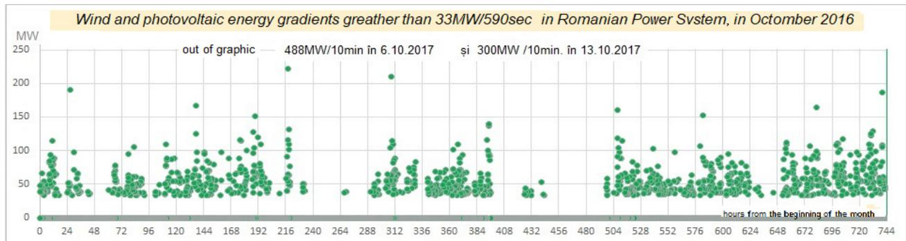
Figure 10. In today SEN, wind and photovoltaic, peaks greater then 33MW inside 590seconds.
