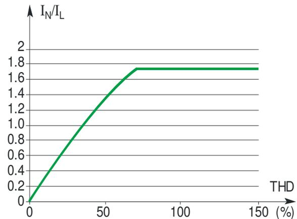
**Fig. 4 Load null conductor at balanced loads**
