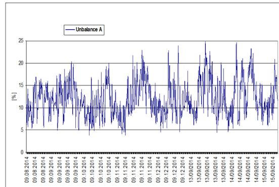
Fig. 1. The variation of the distortion factor through the null conductor in PTab 3 - 20 / 0.4 kV
