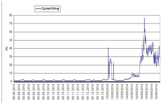
Fig. 5. Current variation through neutral conductor in PTab 2 - 20 / 0.4 kV
