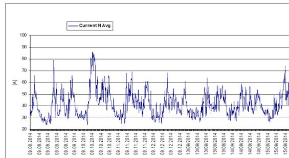
**Fig. 2. The shape of the current through the neutral conductor in PTab 1 - 20 / 0.4 kV**
