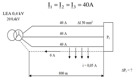
Fig. 7 Symmetric and balanced network
