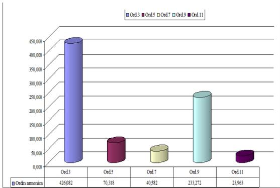
Fig. 4. Spectrum of harmonics through the null conductor in PTab 1 - 20 / 0.4 kV
