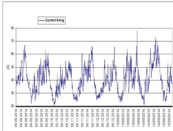
Fig. 8. Current variation through neutral conductor in PTab 3 - 20 / 0.4 kV
