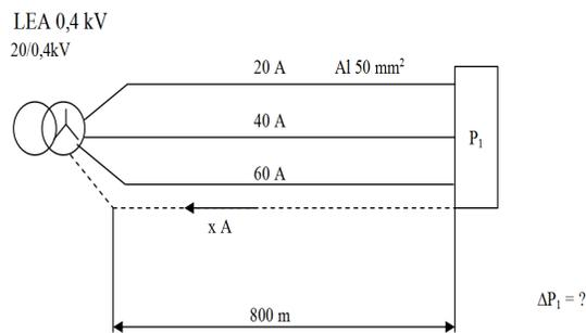
Fig. 8 Unbalanced current network
