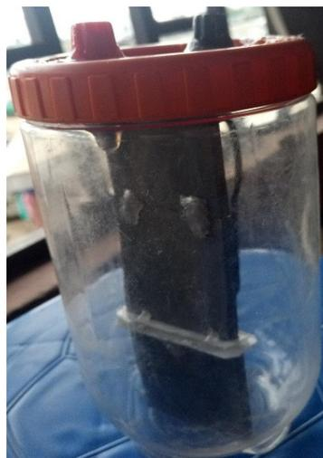
Fig. 2. Picture of the constructed zinc-chlorine cell
