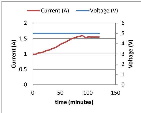
Fig. 3. Graph of charging voltage and current against time for the zinc-chlorine battery
