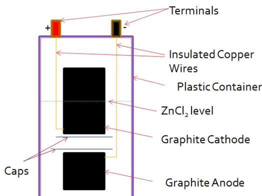
Fig. 1. Schematic diagram of the designed zinc-chlorine cell
