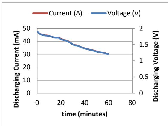
Fig. 4. Graph of discharging voltage and current against time for the zinc-chlorine battery
