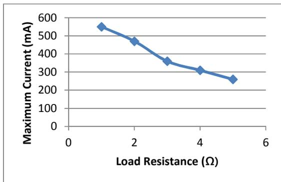
Fig. 5. Graph of Maximum Current against Load Resistance for the zinc-chlorine battery
