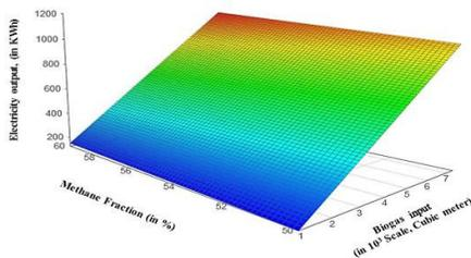
**Fig.7. Electricity output at different biogas input and methane fraction**
